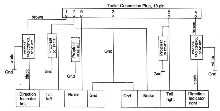
The PROPLAST "PRO-CONTROL" 50 141 012 is necessary for recognizing of Direction Indicator failure.
